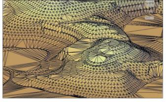
The digital terrain model module enables convenient three dimensional landscape design. The software can read terrain data from 3D scanners or drone cameras and calculate excavation and filling material volumes for different landscape variants.
