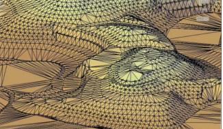
The digital terrain model module enables convenient three dimensional landscape design. The software can read terrain data from 3D scanners or drone cameras and calculate excavation and filling material volumes for different landscape variants.
